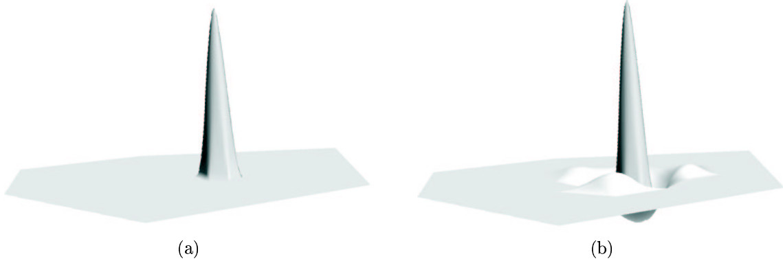
Figure 6. (a) Wavelet function before update is scaling function on finer level. (b) Wavelet function after update.
