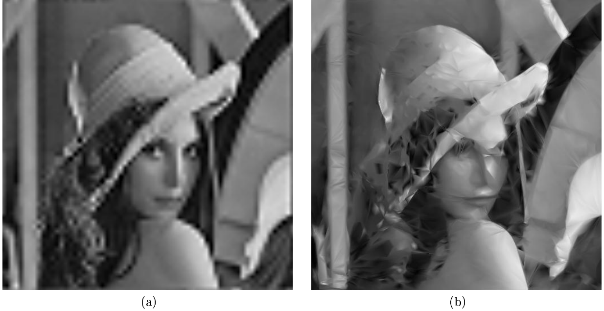
Figure 27: Normal offsets (b), compared to classical wavelets (a). CDF 2,2 wavelets, i.e., linear prediction followed by two-taps update (i.e., update with two coefficients). Normal offsets are directed towards the edges. Triangulation allows for sharper edge reconstruction.
