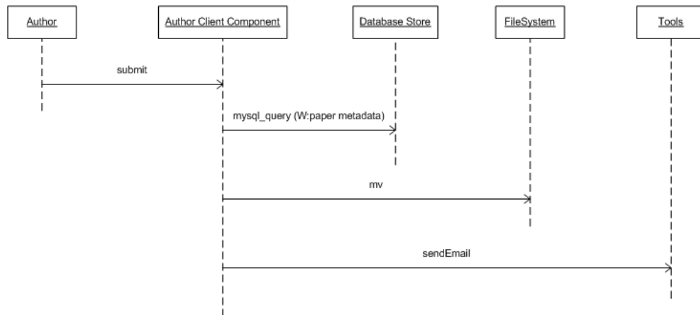
Figure 43: Openconf architecture: sequence diagram of submit paper.
