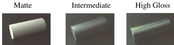
Figure 2: The three coated cylinders.
