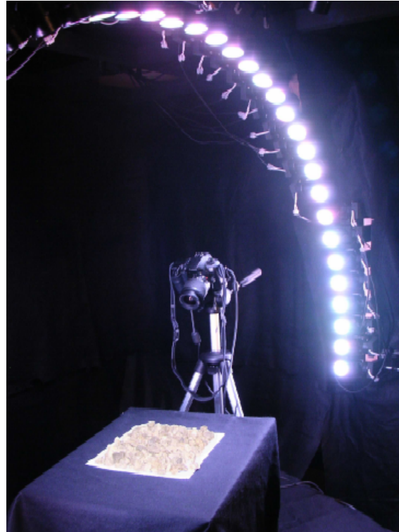
Figure 1: The setup for our data acquisition. The scene, a set of stones, and the camera are placed on a turntable. A semi-circular brace with 40 light sources is mounted over the turntable. By rotating the turntable 180 degrees in 32 steps and switching on one light source at a time, the object can be illuminated from 64 \times 20 regularly sampled directions.
