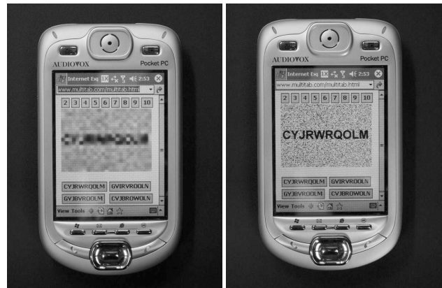
Figure 1: Snapshot of the PDA with the multi-tab interface that allows users to select an arbitrary fidelity level. The left and right snapshots show the same image at low and high fidelity, respectively.
